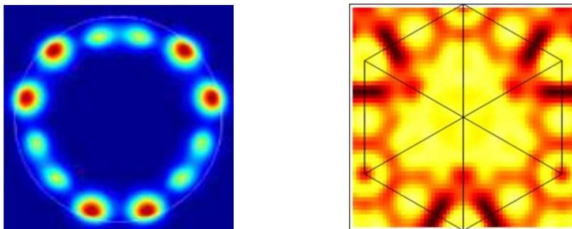
Figure 1: Left: Wavefunction of a TMD based Nanobubble; Right: Electron population in MoS<sub>2</sub>, 400 fs after optical excitation
